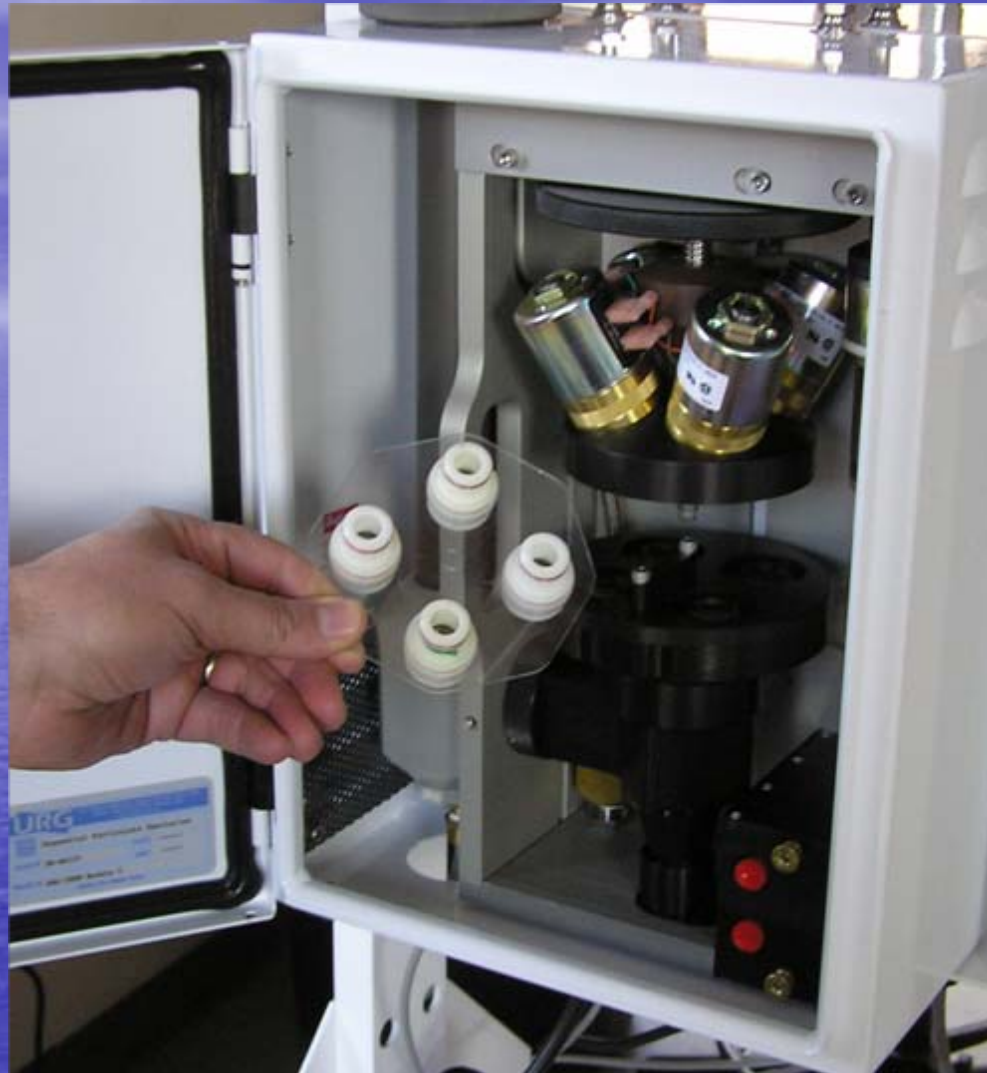
URG 3000N Aerosol Sampler Module with Removable Filter Cassette and Four Cartridges.
