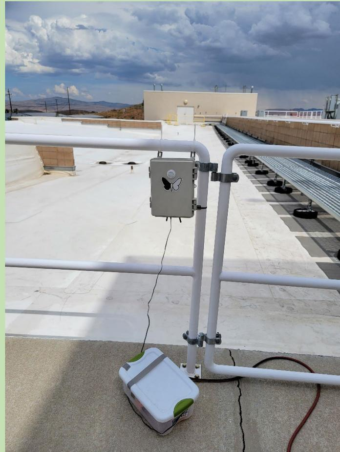
DST ObservAir → BC (880 nm) and BrC (405 nm)
