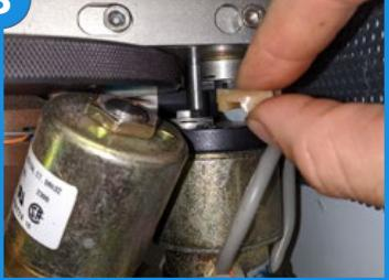
Remove the old plastic coupler and place the new one in. Make sure to center it on the metal hub.
