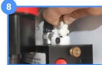
Re-connect the hoses to the electronics box.
