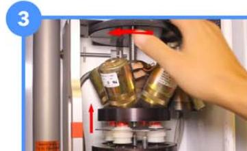
For the A, B, and C modules spin the hand wheel to the left to raise the manifold.
