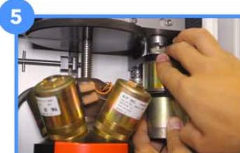
If the motor starts to work again it can be reengaged with the hand wheel. Pivot the motor assembly back to its original location.
