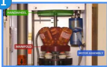
Locate the motor assembly in the module
