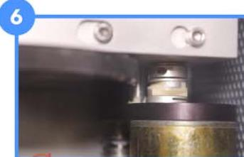
Rotate the hand wheel until the coupling snaps into alignment.
