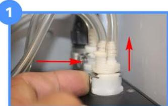
Disconnect the Orifice (ORI) and Cyclone (CYC) hoses by depressing the metal clasp and pulling on the hose.
