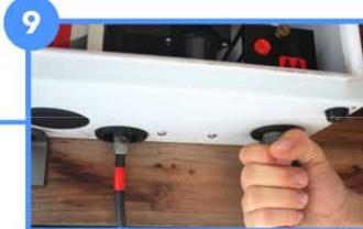
Re-connect the bottom grey module cable.
