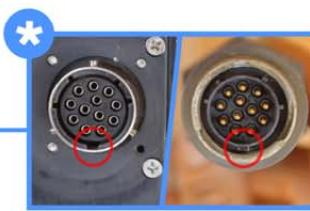
(line up the key and keyway when connecting the electronic connectors)
