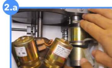
A gentle wiggle may be required to slide the assembly up or down.
