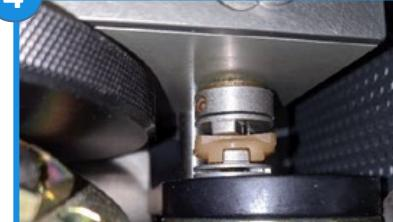
If the plastic motor coupler does not line up with the upper hub, use the hand wheel to put it into place
