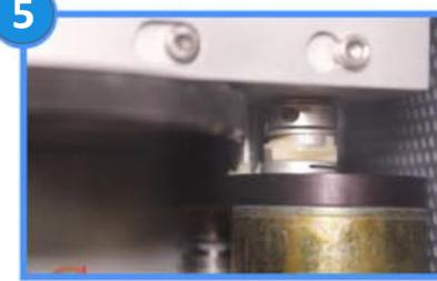
The motor should slide into place and the upper and lower hubs should fit securely into the plastic motor coupler
