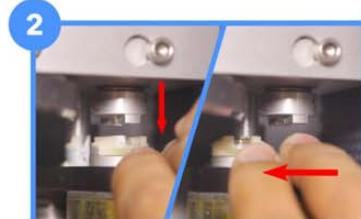
Separate the motor assembly from the coupling sliding the assembly down. Then pivot it towards the hand wheel.
