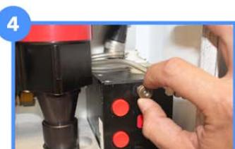
Loosen the brass knobs located on the black electronics box.
