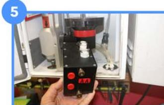
Remove old electronics box and insert the new box.
