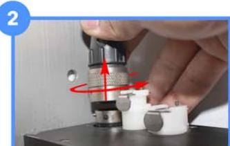
Disconnect the grey cable located on top of the box by turning the metal collar counter-clockwise.
