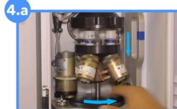
The spinning direction to raise and lower the manifold is opposite for the D module.
