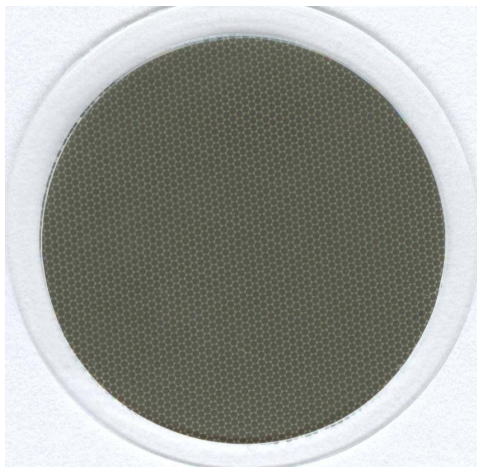
Figure 1.8. Filter sample collected using detached screen cassette.
