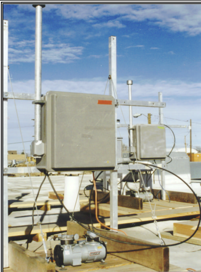
Figure 3. A four-module IMPROVE sampler, installed and operating in Denver, Colorado.
