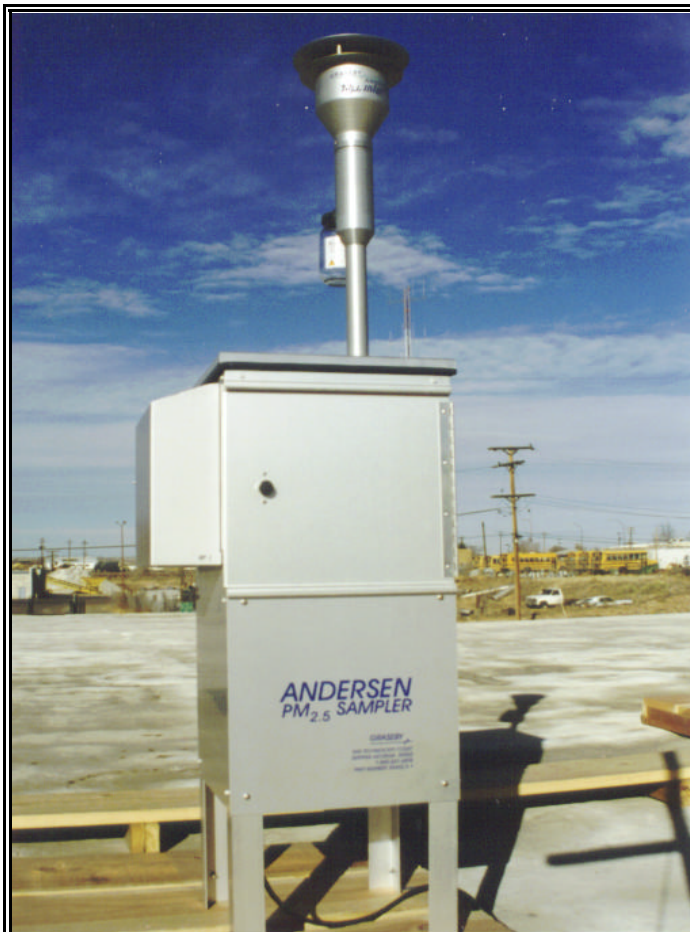
Figure 2. A Federal Reference Method (FRM) sampler, installed and operating in Denver, Colorado.
