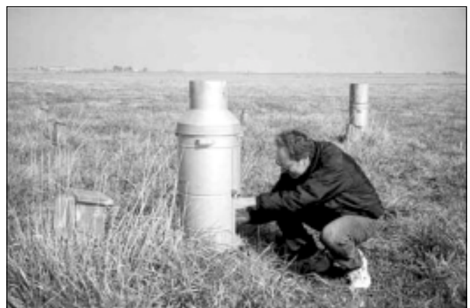
Mike Snider, with the Illinois State Water Survey, services a National Acid Deposition Program Belfort Recording Rain Gauge. Mike also services an IMPROVE aerosol sampler at the Bondville site.
