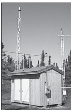
At left, the air quality monitoring shelter in Ambler, AK, with IMPROVE aerosol sampler, CASTNet filter-pack tower, and meteorological tower. Wet deposition and mercury deposition samplers are nearby.
