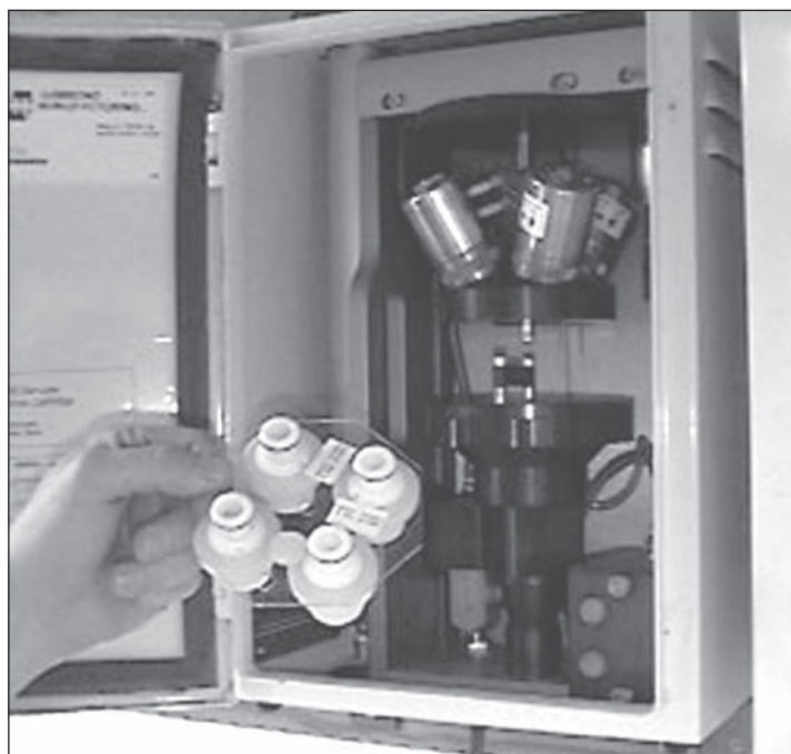
Figure 3. Example IMPROVE aerosol sampler module with removable filter cassette and four cartridges. Each cartridge holds filter media which carbon from ambient air is deposited onto. In the STN program, only one of the cartridges will hold a filter and the other three will hold a blank. The operator will change the filter cartridges every 3 or 6 days, depending upon individual station protocols.
