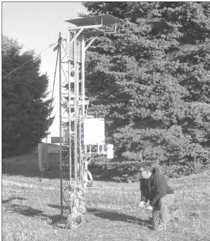
Figure 2. Field Specialist Dave Beichley demonstrates the nephelometer elevator system. The instrument is lowered to ground-level via a manual hand crank for servicing. The unit is then cranked back to the top of the tower for operational monitoring.
