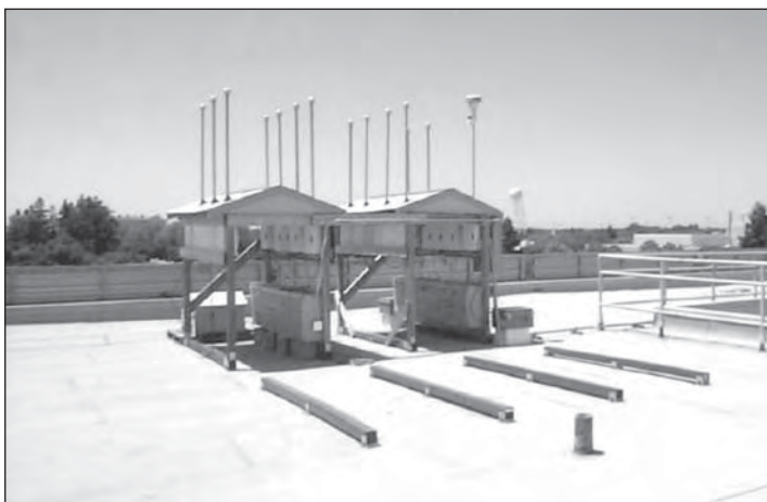
Figure 1. The new UC-Davis aerosol sampler test site, located atop the engineering building, uses various operational configurations of modules, which are used for numerous tests and comparison studies. A third sampler shelter was added shortly after this photo was taken.
