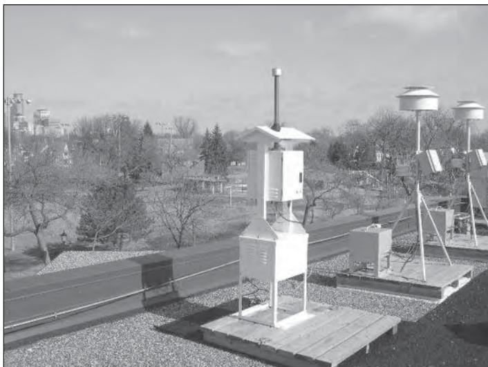
The URG3000N carbon sampler is based on the IMPROVE Version II sampler (Module C), with a few operational differences. Early analyses between two collocated samplers show excellent correlation in organic carbon and elemental carbon. The above photo is the URG3000N carbon sampler operating at the CSN Minneapolis, MN, monitoring site. Two SASS samplers are pictured in the photo's right.
