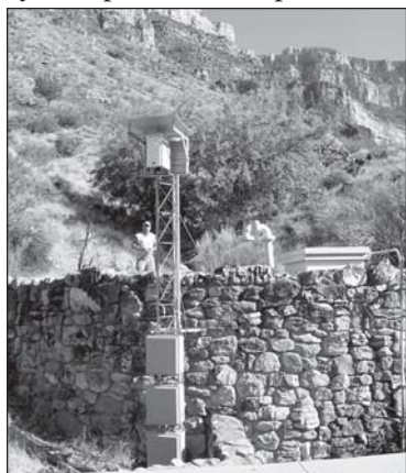
The nephelometer at Indian Gardens in Grand Canyon National Park, Arizona, is configured with an automatic span calibration system.
