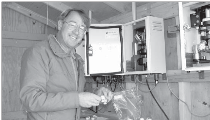
IMPROVE site operator Charles Conner maintains the IMPROVE sampler, a nephelometer, and various other air/meteorology instrumentation at Organ Pipe Cactus National Monument, Arizona.
