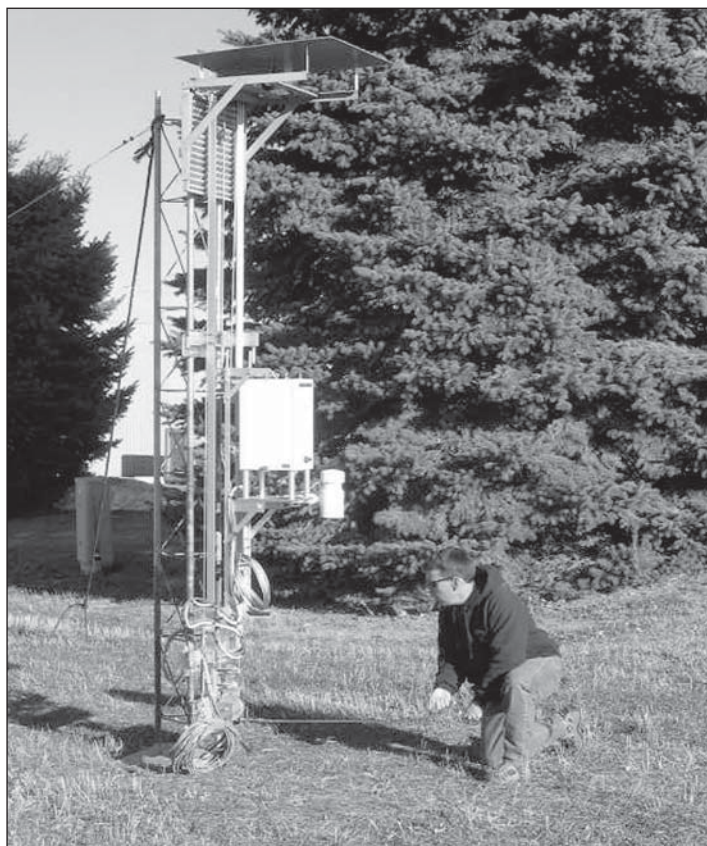
The nephelometer tower elevator is operated by hand cranking a winch and pulley system. The operator lowers the nephelometer to a safe servicing height, and again raises the instrument to the top of the tower for routine operation.
