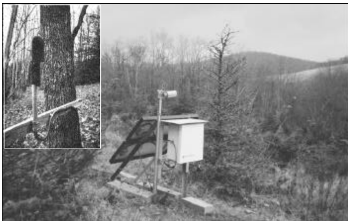
The sound monitoring system at Great Smoky Mountains National Park - Purchase Knob, consists of a processing station and a microphone. The microphone (inset) is located approximately 100' from the processing station in a stand of trees.
