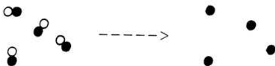
Figure 24-42 Two distinct possibilities for the response of an aerosol to the removal of a constituent. The model aerosols are composed of two species, one of which (drawn in white) is eliminated by controlling emissions. The initial aerosols have identical size-resolved chemical compositions, but the remaining aerosols consist of doublets in the external mixture model, singlets in the internal mixture model.
