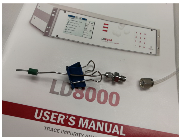
Figure 3-3. Pictures of: (a) probe connecting LD8000 to carbon analyzer; and (b) measurement of trace level O 2 in a carbon analyzer.
