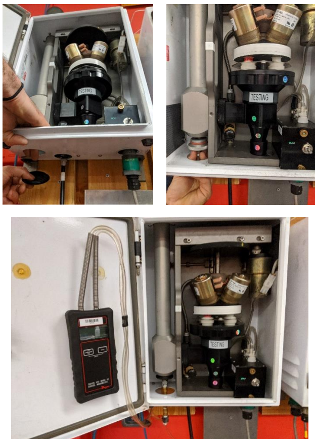
Figure 1. Removing the plastic cap and stack plug and inserting the probe into the tee.
