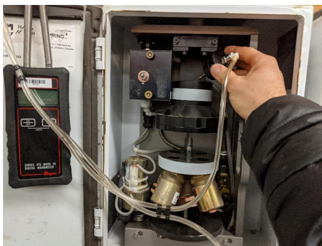
Figure 7. Inserting the flow check probe into the 4D Module.
