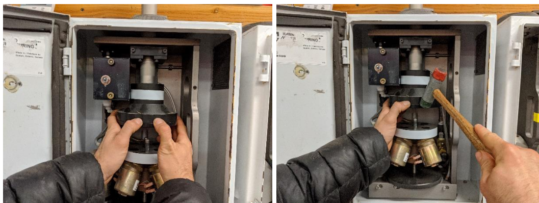
Figure 8. Removing the bottom lid of 4D Module funnel.
