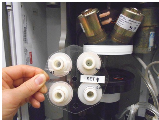
Figure 2. Calibration system with Definer 220.
