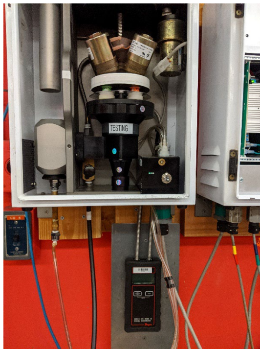
Figure 6. Calibration system with magnehelic flow meter.
