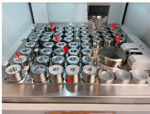
Figure 2. Sample changer compartment with trays.
